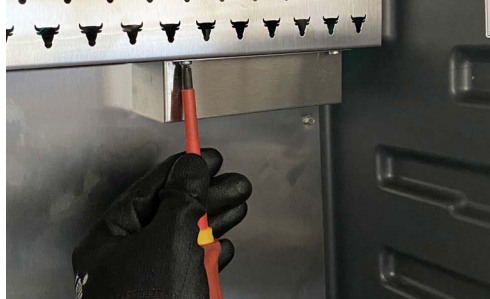
5. Unscrew the cover with a Phillips screwdriver.
