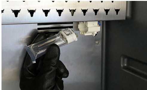
7. Pull out the old UVC bulb carefully then carefully insert the replacement UVC bulb. Do not remove the outer plastic cover of the UVC replacement bulb.
