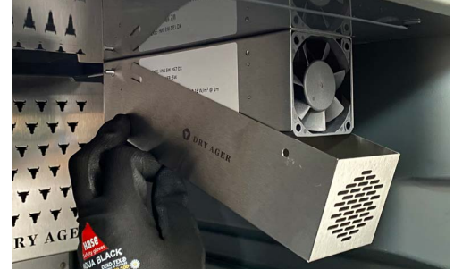
6. Slide the cover out of the rear holding.
